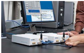
1. Modern SDRs have the ability to link with other SDRs for test & measurement and research & development purposes. (Courtesy of National Instruments)
